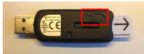
Figure 11: "Correct insertion of the chipcard"
