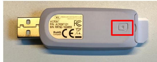
Figure 15: "Correct insertion of the chipcard"
