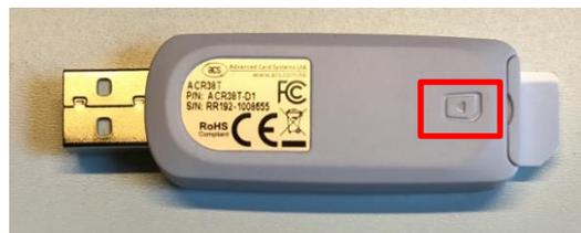
Figure 15: "Correct insertion of the chipcard"
