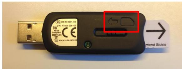
Figure 11: "Correct insertion of the chipcard"
